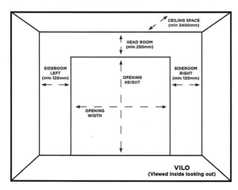
**Step One:** Measure the width of the opening at its widest point. This is the distance between the left and right sides of the finished door opening.
